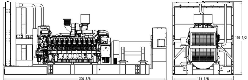
Drawing above for illustration purposes only, based on standard open power 480 volt generator. Lengths may vary with other voltages.
